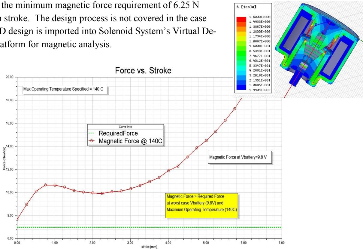
This design satisfies the force requirements at the Maximum Ambient Temperature of 140C with the Minimum Supply Voltage of 9.8 V. The design needs to be analyzed for the other two thermal conditions to verify that the force requirements are still satisfied.
