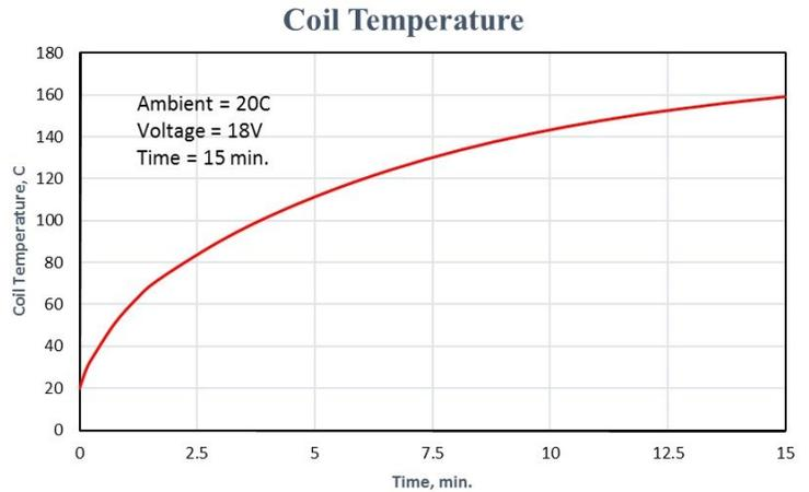
The Coil temperature reaches a temperature of 159 C after 15 minutes. This temperature is input back into the magnetic analysis to analyze the force vs stroke performance. The graph below shows that the force requirements are still satisfied at 159C. If the force requirements were not met for this thermal condition a redesign would be required.
