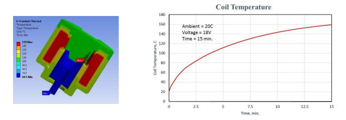
The Coil temperature reaches a temperature of 159 C after 15 minutes. This temperature is input back into the magnetic analysis to analyze the force vs stroke performance. The graph below shows that the force requirements are still satisfied at 159C. If the force requirements were not met for this thermal condition a redesign would be required.
